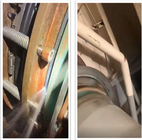
Figure 1: Sea water discharging through seal face
